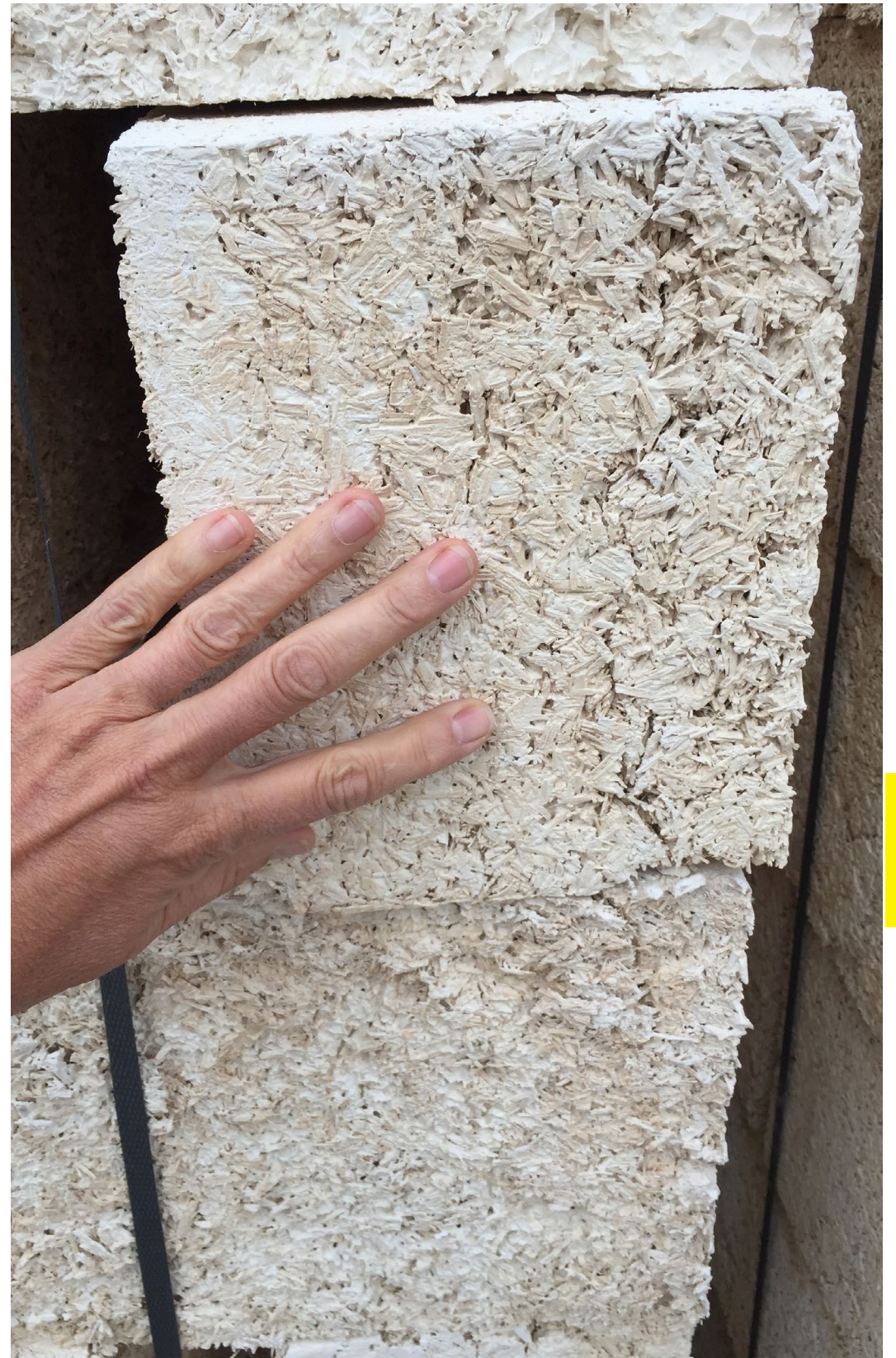
Fig 6.11 Hemp and lime blocks + mortar, Puglia, Italy
