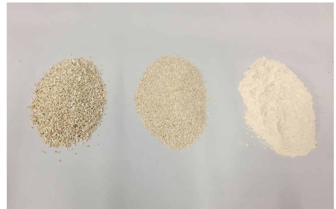
Fig 4.8 Different granular sizes of crushed limestone
