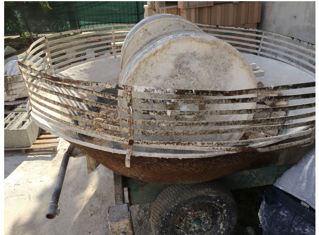
Fig 1.13 Crushing hemp and line blocks for reuse
