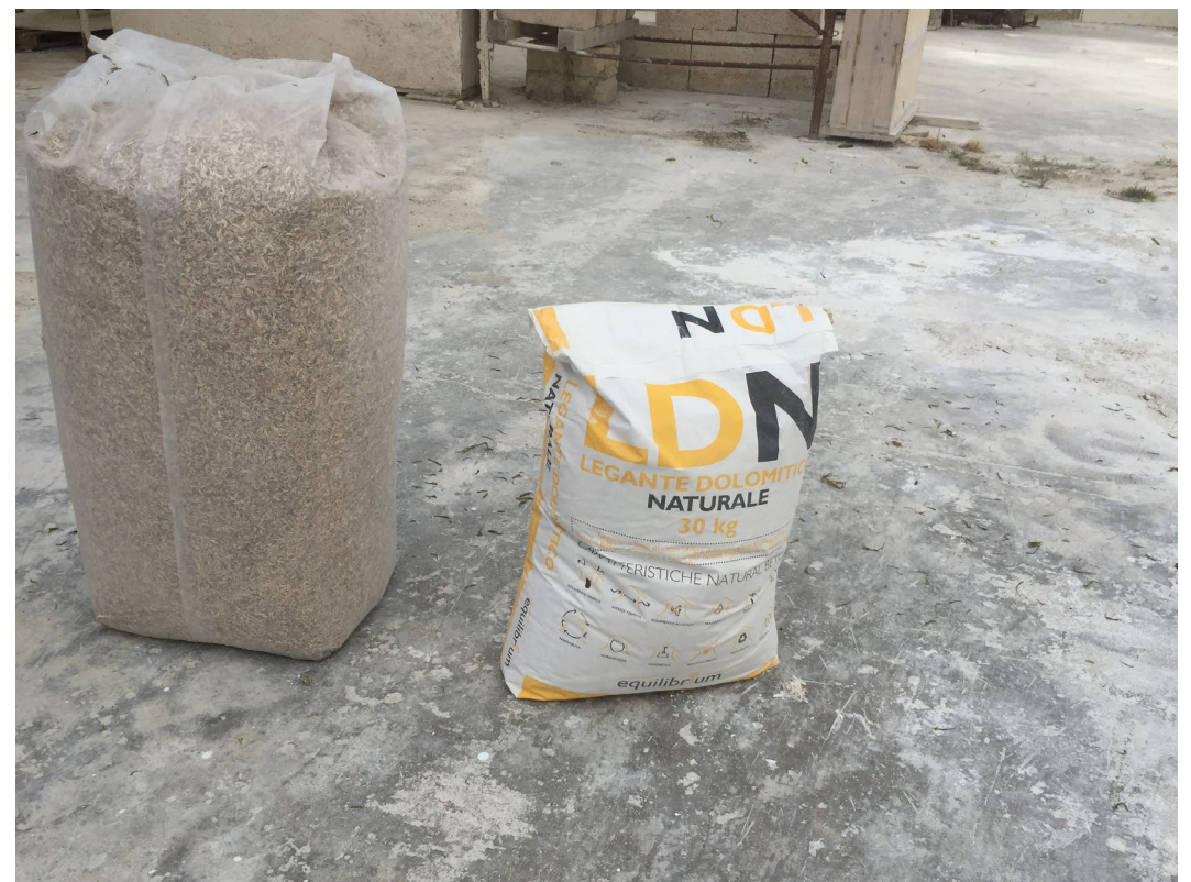
Fig 1.14 Hemp hurd and lime binder
