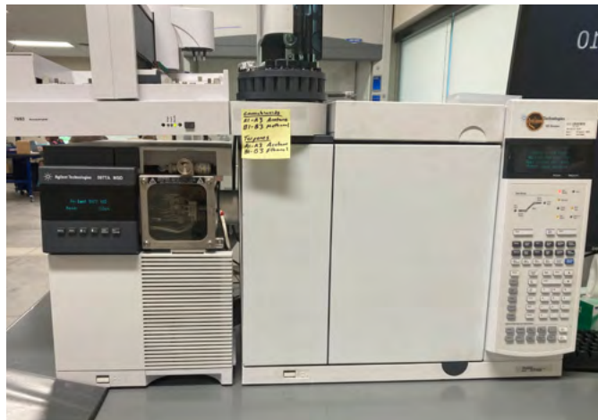
Equipment to measure cannabinoids, terpenes, and other compounds from the C. sativa plant. Left: High performance liquid chromatography (HPLC). Right: gas chromatography mass spectrometer (GC-MS). Photos: Daniela Vergara
