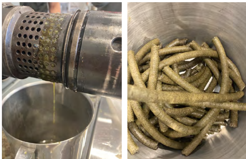
Seed oil extracted using a screw press (left). After the oil is extracted from the hemp seeds, a press cake is extruded from the screw press (right). Photos: Daniela Vergara, CCE
