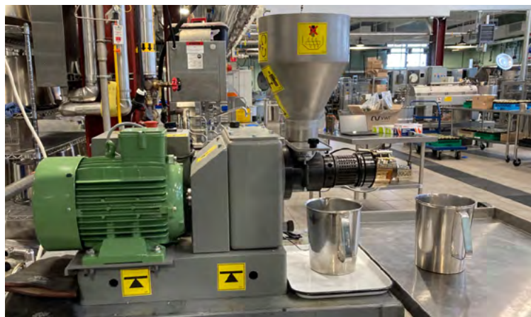
Screw press to process hemp seed oil at Cornell’s AgriTech Food Science Pilot Processing Plant. Photo: Daniela Vergara, CCE
