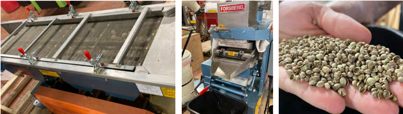
A shaker table separates seeds using mesh screens (left), a destoner for separating based on weight (center), and hulled hemp hearts (right). Photos: Daniela Vergara, CCE
