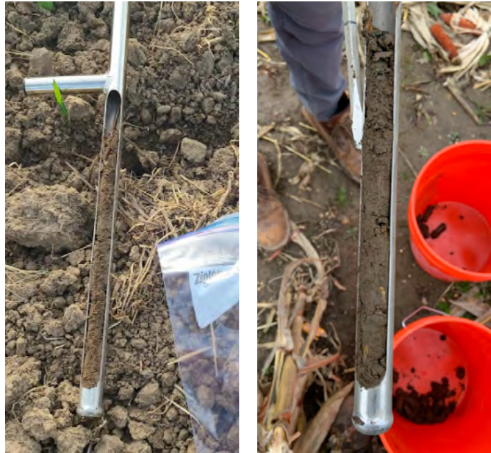
A 12-inch (30 cm) soil probe core taken in the spring before planting (left) and fall after harvest (right). Ten cores were combined in a gallon Ziplock bag (left) or buckets (right) to represent a 1-acre field.
