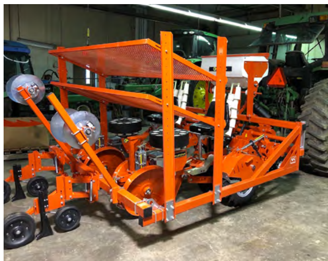
Transplanter machine allowing consistent space between plants and a better packing. Photo: Larry Smart, Cornell
