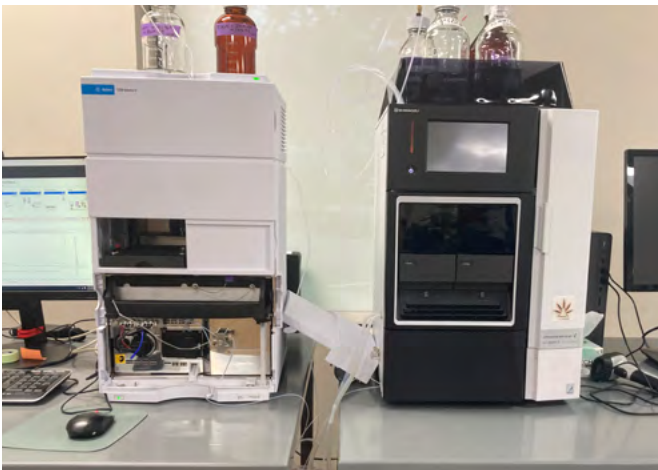
Equipment to measure cannabinoids, terpenes, and other compounds from the C. sativa plant. Left: High performance liquid chromatography (HPLC). Right: gas chromatography mass spectrometer (GC-MS). Photos: Daniela Vergara
